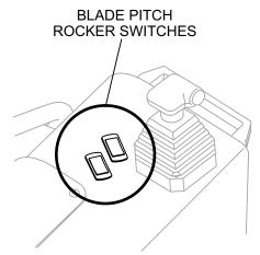
Figure 16. Blade Pitch Control Rocker Switches Location
